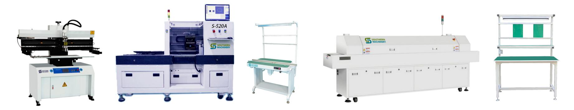
Semi-Auto Screen Printer  $\rightarrow$  Semi-Auto Pick and Place  $\rightarrow$  Buffer Conveyor  $\rightarrow$  Reflow Oven  $\rightarrow$  Buffer Conveyor 3000mm 1500mm 1200mm 2000mm 1500mm
