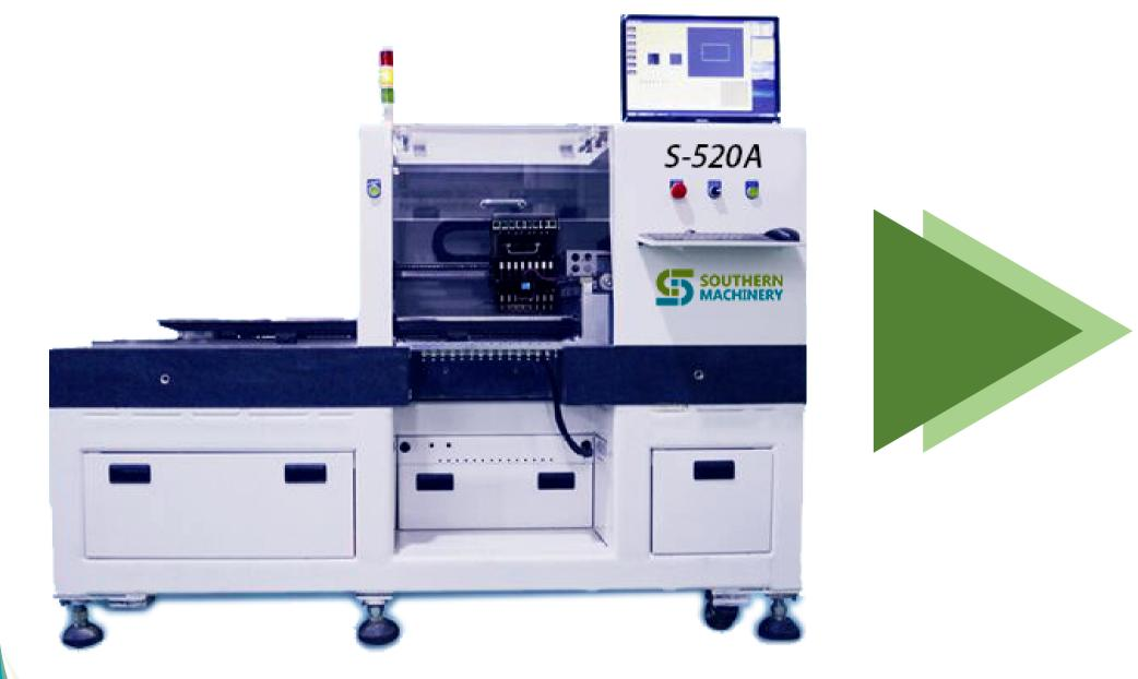
• Actual placement speed to **35,000** mph for LED tube light.
